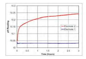
Electrode 1 has been properly cleaned before calibration. Electrode 2 has not been properly cleaned.
